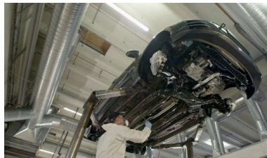
13. Apply underbody coating
